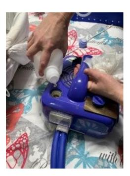
7. Switch the cooling unit on by pressing the on/off button. Press the down arrow until it shows 8 degrees and then press enter. (The unit takes about 45mins to become cool)
