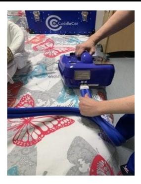
4.Plug the cooling pad connectors into the end of the hose. You should hear a click.
